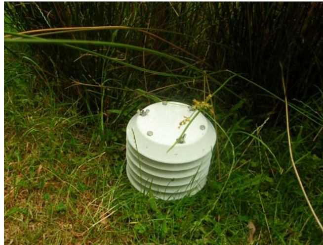
Figure 8. Instrumentation deployed to measure air temperature during the study.
