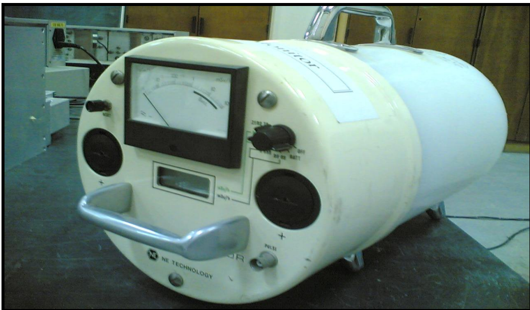
Figure 2.2: Neutron dosimeter detector (NM2B), Serial No. 433[67].
