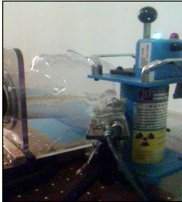
Figure 4.2: Head phantom containing the tumour vessel in the lateral position.
