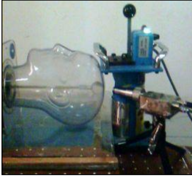
Figure 4.22: Head phantom containing tumour vessel in the vertex position.
