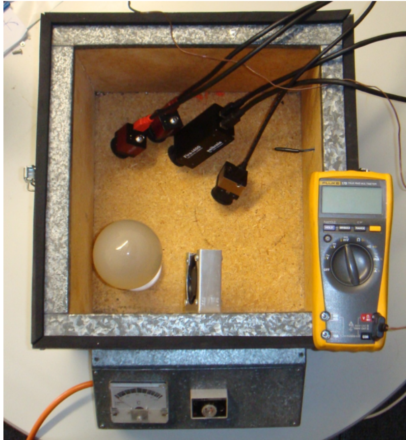
Figure 3.25 The temperature-controlled thermal chamber with the 4 cameras under test.
