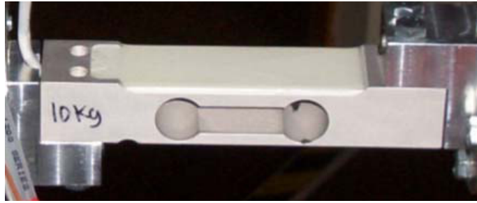
Figure 3.12 Load cell used in the cutting trials.
