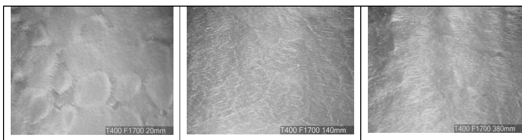
Figure 3.22. Cutting force/surface finish relationship for S-grade EPS (5A – 0.0283m/s).
