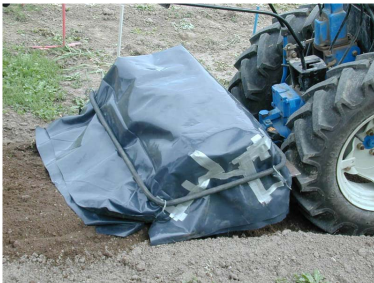
Plate A10-3. S.E.P. rotary hoe with Perspex shield covered during cultivation.
