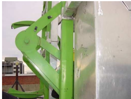
Figure 3.22. Y axis frame pivot without bottom strengthening gusset.
