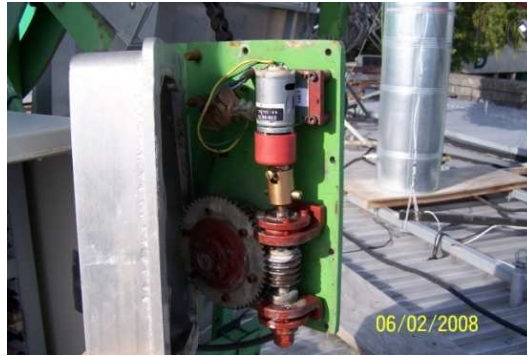
Figure 4.1. The Y axis drive & DC motor, final output worm-drive and mounting assembly.
