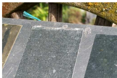
Figure 8.20 c. Clear Dome substrate top edge lifting.
