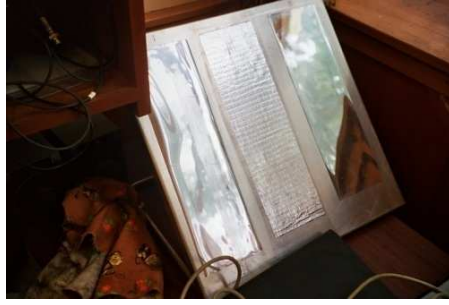
Figure 8.7. TP#3 in January 2004, showing the lifting of the 3M panels on the left side of the 3M substrate.
