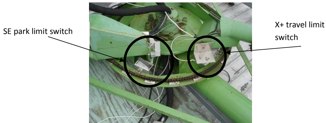
Figure 7.1. The X+ travel limit switch and the SE park limit switch.
