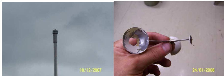
Figure 9.8. Wind anemometer mast and cups after a weather bomb in late 2007.
