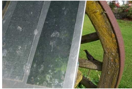
Figure 8.20 d. Nielsen substrate, showing weathering only with no other damage.
