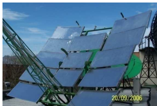
Figure 11.2 c. The polished state of the mirrors in September 2006.
