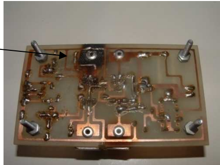
Figure 5.6 Drive control interface circuit board –track side.
