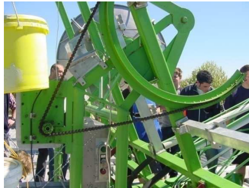
Figure 3.5. The Y axis support frame drive mechanism.
