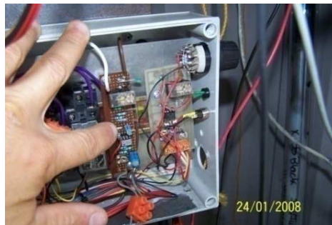
Figure 5.16. Flow and Over pressure circuitry for CP.
