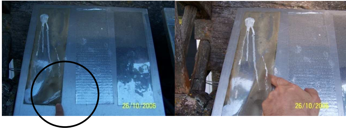
Figures 8.27 a & b. TP#2 enlarged taken 26 th October 2006, showing total failure of the 3M substrate (follow the finger).
