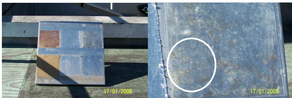
Figure 8.59 a & b show AP#1 and the complete failure of 3M substrate and slight tarnishing on the Nielsen substrate.
