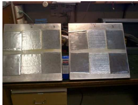
Figure 8.39. The completed AP#1 and AP#2 test panels following the gluing process – no edge sealing has yet occurred.
