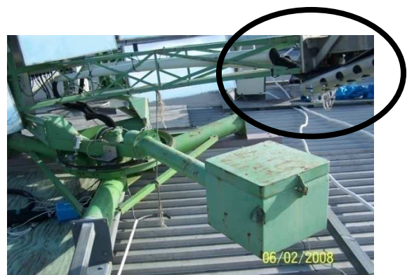
Figures 3.6 a and b. Showing two bottom attachment points for the Y axis and Y axis boom respectively.
