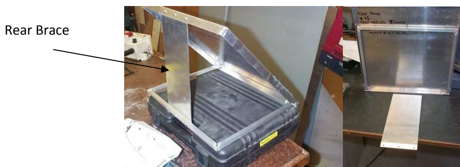
Figure 8.38 a & b. AP#1 rear aluminium strip bracing. (13 th November 2003).
