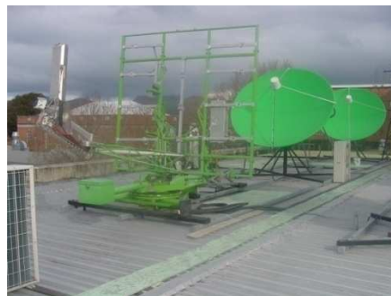
Figure 3.16. The Y axis sub-frame with additional mounting supports for the mirror's ball joints.
