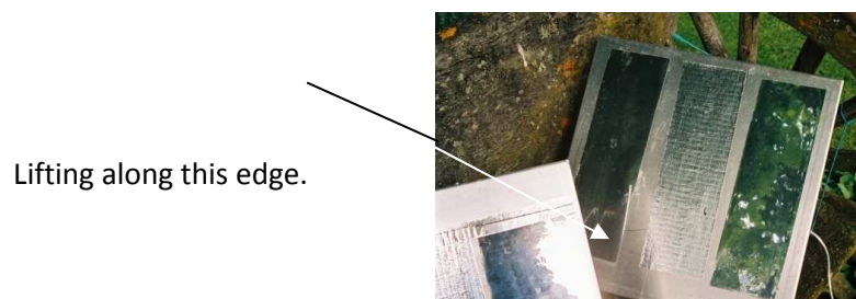
Figure 8.11. TP#2 in November 2004, with all mirror substrates all intact, but some lifting on the 3M substrate right lower edge.
