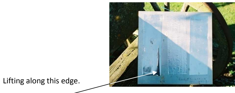
Figure 8.9. TP#2 in June 2004, showing all the mirror substrates still intact, (but with signs of lifting on the 3M panel (right side edge)) and showing signs of weathering, i.e. all substrates are dull.
