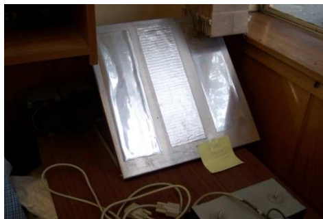
Figure 8.25. TP#3 taken 25 th May 2006, showing only limited deterioration with some lifting of the 3M substrate side edges.
