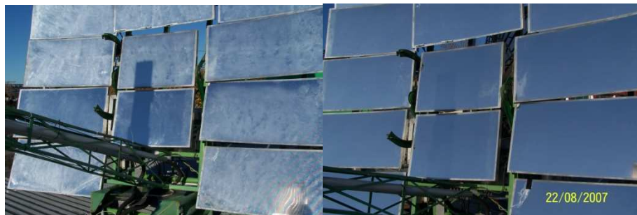
Figure 8.66 a & b. 3M mirror substrate before (a) and after (b) polishing.
