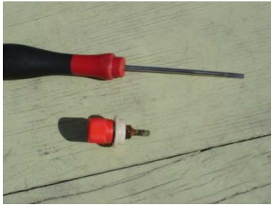
Figure 5.15 a & b. a) The rusted flow sensor from the CP outlet header, b) the inline magnetic float replacement.
