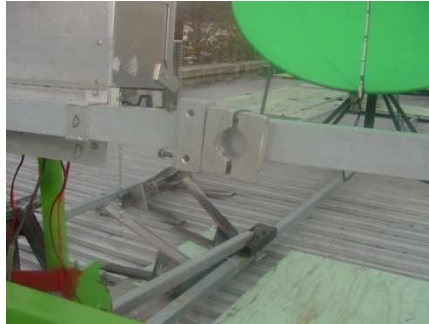
Figure 3.17. The mounting support and mirror ball joint receptacle.
