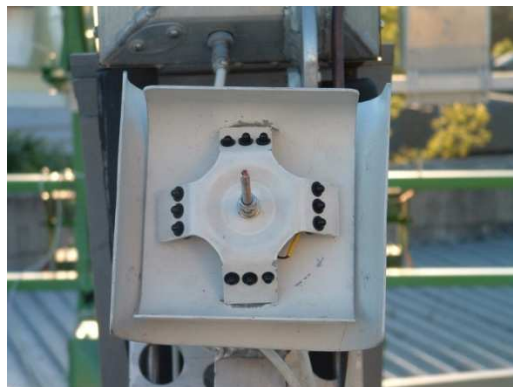
Figure 3.14. Auto-tracking sensor head arrangement.
