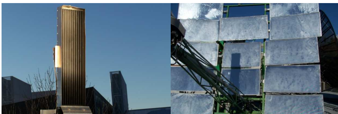
Figure 11.9 a & b. The target with dirty or unpolished mirrors, 20 th June 2006.
