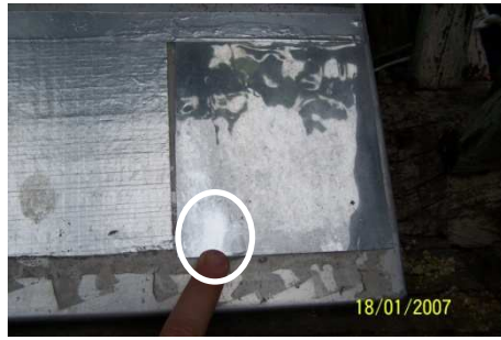
Figure 8.56 c. AP#2 taken January 2007, with a light cleaning of a small area of the Nielsen substrate.
