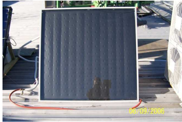
Figure 10.17. Matt black folded stainless steel glazed flat panel under test 6 th September 2006.
