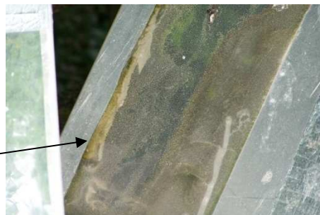
Figure 8.20 b. Tarnishing of left edge of 3M panel.
