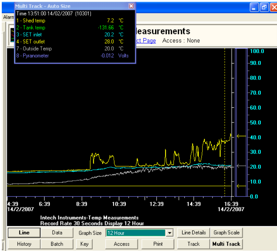
Figure 11.5. The peak temperature gain for the 14 th February was 43.4 °C, the average temperature gain was 21.6 °C. The SET operated for 6 hours on this day.
