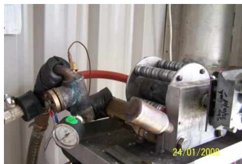
Figure 5.12. CP mounting assembly for peristaltic pump.
