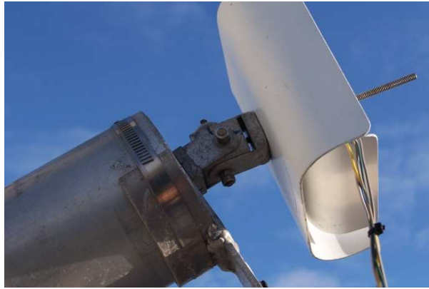
Figure 3.13. Auto-tracking target and knuckle adjustment.
