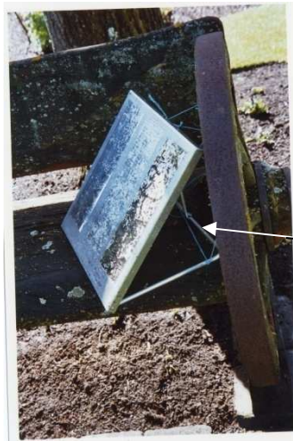
Figure 8.1. Mirror edge fold-back for correct angle support.
