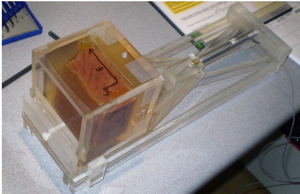
Figure 3.7: The completed beef muscle phantom before imaging. The phantom box is connected to the supporting tray in one particular orientation with nylon screws. The tray is in turn coupled to the actuator.
