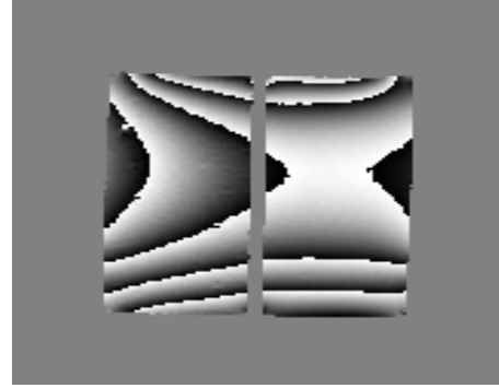
Phase image with aluminium alloy actuator
