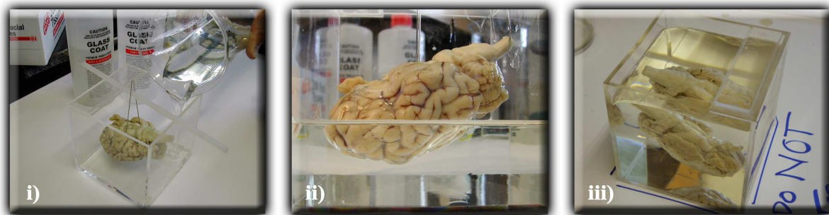
Figure 3.8: From left to right: i) The brain is suspended by stainless steel wires while the first batch of epoxy resin is poured in. ii) The resin is allowed to harden, thus supporting the brain and allowing for removal of the wires. iii) Following several further resin pours, the brain is entirely encased. The epoxy resin offers excellent optical clarity.
