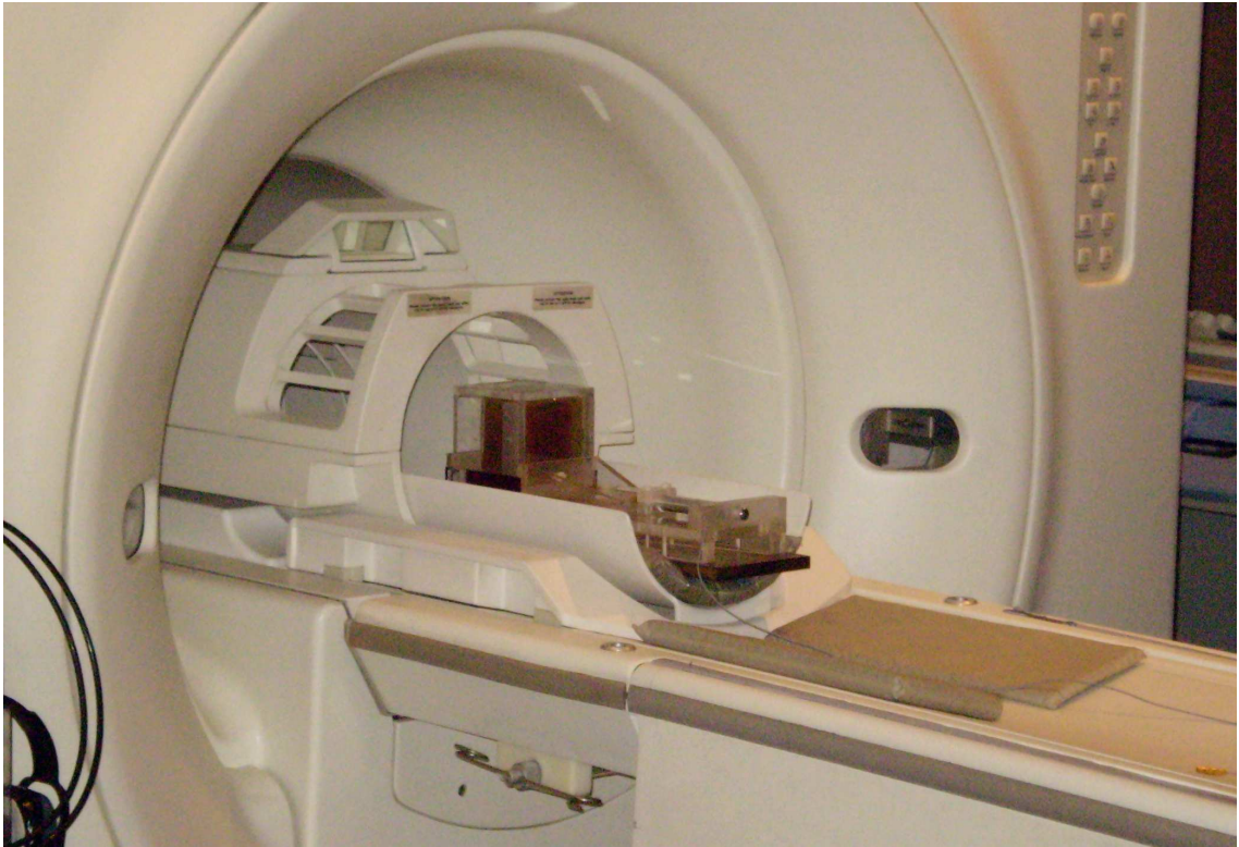
Figure 3.3: The phantom actuation apparatus sitting on top of the scan table before insertion into the bore of the scanner. The head coil used is in place, but moved so the phantom can be viewed; a 3D-orientable excised muscle phantom is coupled to the actuator.
