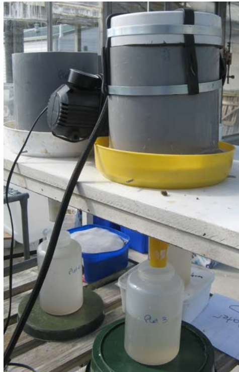
Figure 3.4 Air compressor system to remove excess moisture from soil cores after each leaching event.
