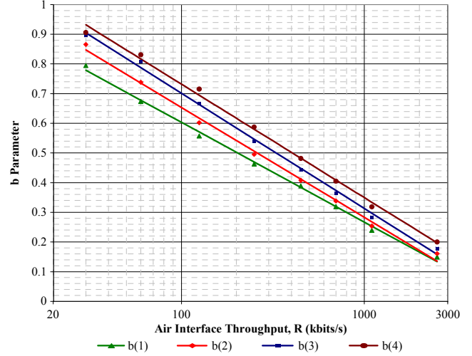
Figure 4. Fit of web only simulation results to the relationship between R and b defined in (8), for all service classes.
