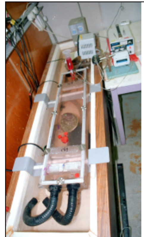
Figure 4.6: Photograph showing flume respirometer in operation.
