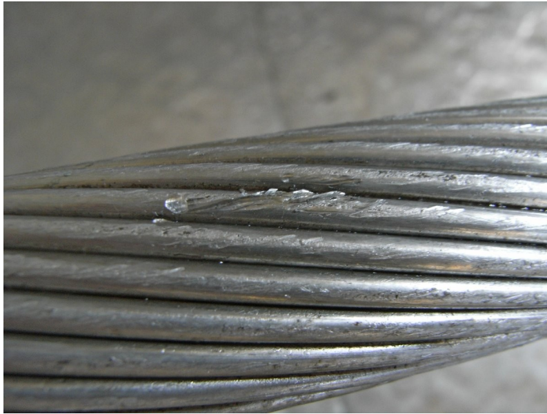
Figure 4 - 'Used Midal Bungama' conductor with a jagged scratch which corona flared from.
