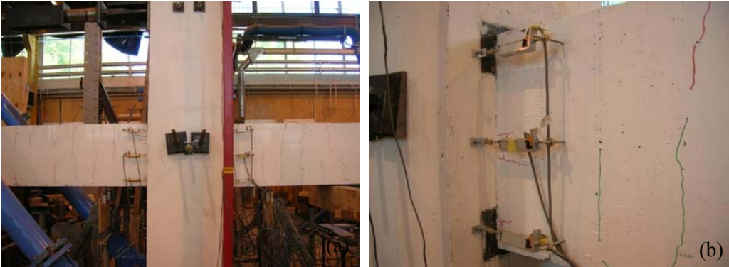
Figure 7: Photographs of the specimen after uni-directional QS testing: (a) the specimen at approximately 3 percent drift; (b) the west beam after completion of testing.
