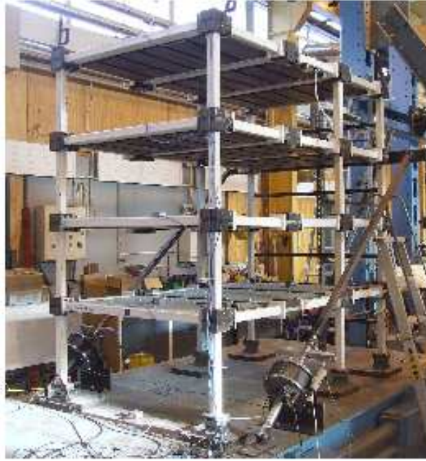
Figure 2. Photograph of test structure on the shake table with the devices installed.
