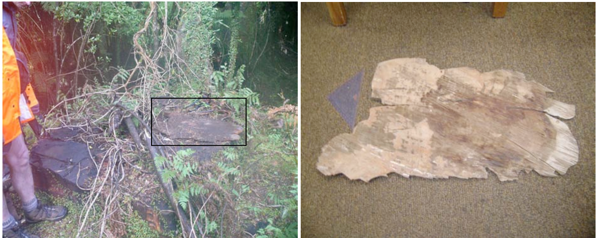
Figure 46: Piece of Matai on site and after drying and treatment.
