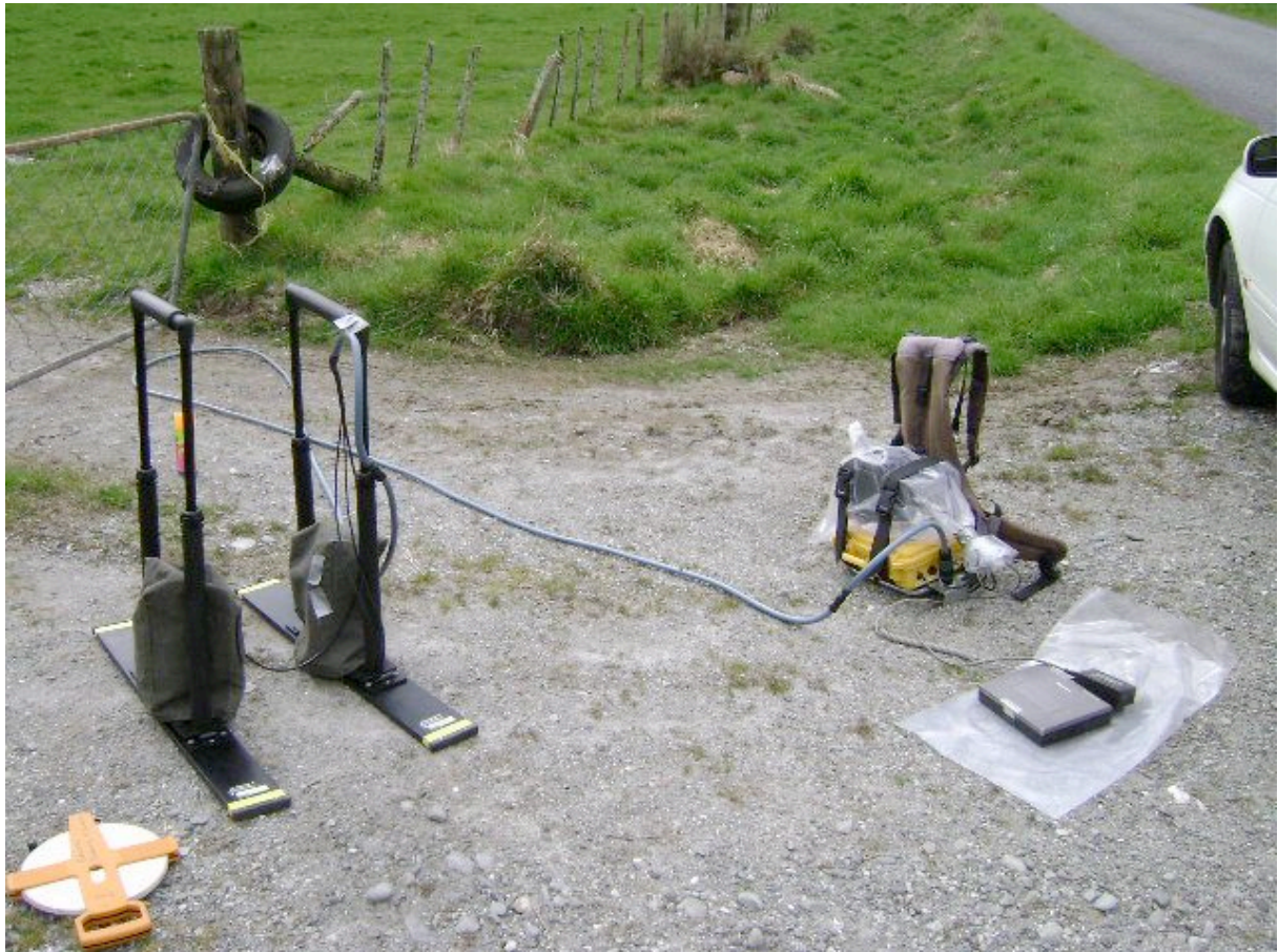
Figure 28: pulseEKKO 100 GPR apparatus.
