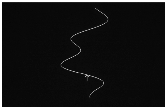
Figure 6-1 A screenshot depicting the random-preview target waveform used for the CTT. Subjects were instructed to keep the arrow-head of the cursor (which could only move horizontally) on the target waveform as closely as possible.
