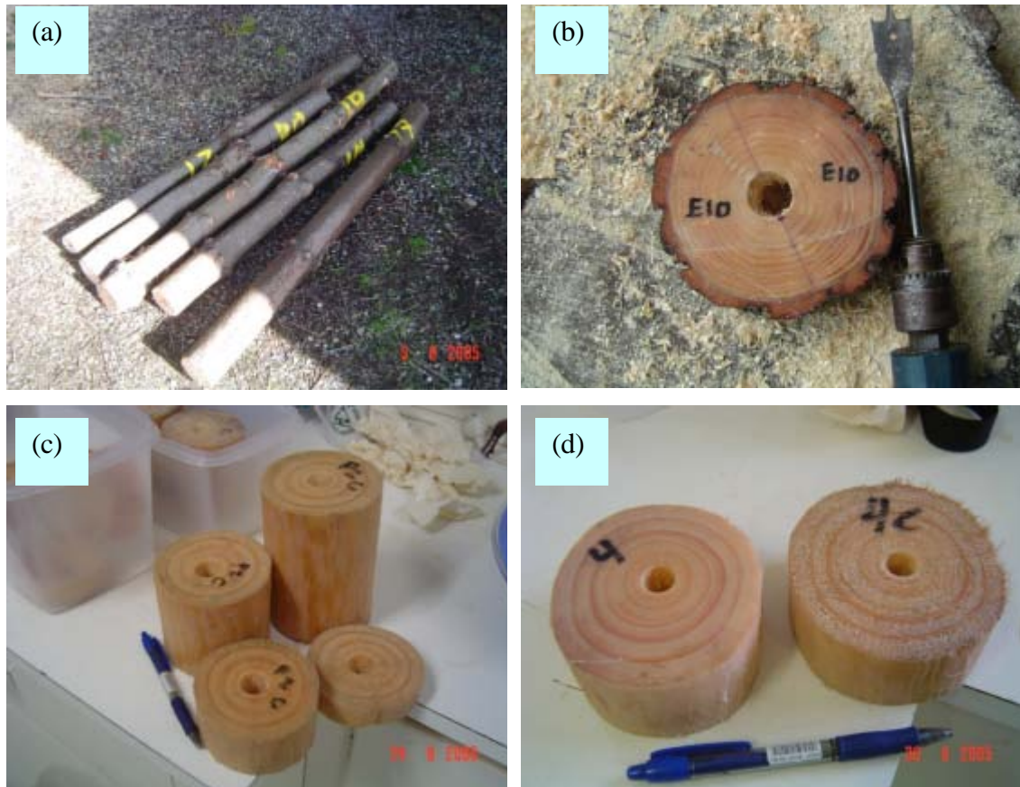
Figure 3-2. Details of sample processing: a) fresh logs, b) removal of dry centre with drill and speedbore, c) samples of the four thicknesses tested, d) cross sections showing cutting methods, fine dropsaw on the left and chainsaw on the right
