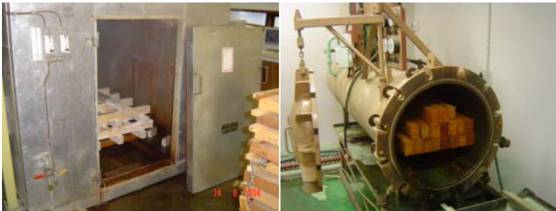
Figure 2-1. Kiln used for temperature conditioning and for some moisture levels (left); and preservation cylinder for saturation (right)
