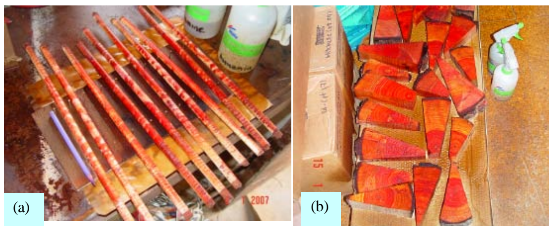
Figure 4-4. a) Bark-to-bark 12 mm cores; and (b) pith-to-bark wedges immediately after staining to detect heartwood (wedges shown before dressing to separate sapwood and heartwood sections)
