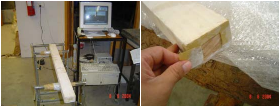
Figure 2-3. Full set up for acoustic measurements with WoodSpec (left); and windows opened at the end of the boards for launching and detection of acoustic signal (right)
