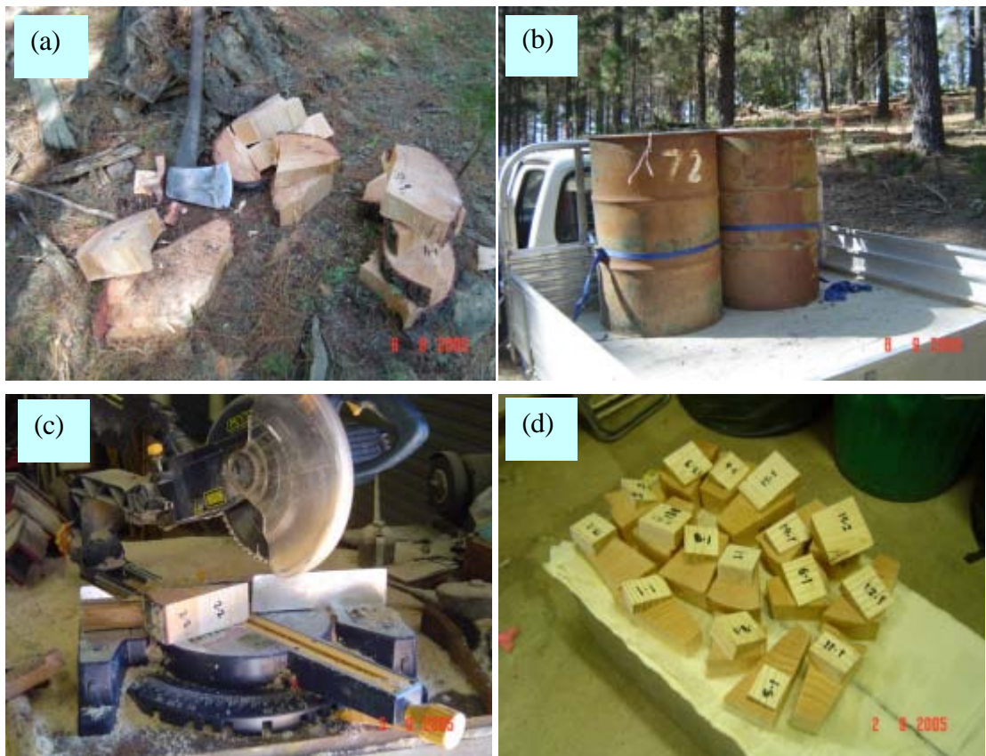
Figure 3-4. Details of sample processing for mature trees material: a) Sections of disks, b) Transportation in drums with water, c) Portable dropsaw with thin kerf, d) Heartwood (top) and sapwood (below) dropsaw samples after green measurements
