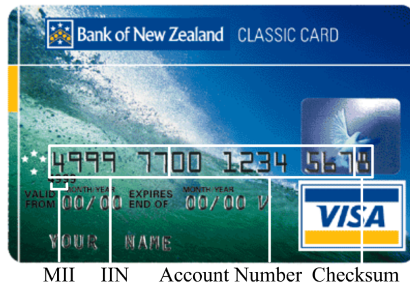
Figure 2.3: The first digit is the Major Industry Identifier (MII). The first six digits (including the MII) is the Issuer Identifier Number (IIN). The seventh to second to last digit is the account number. The final number is a checksum using the Luhn algorithm. Image is from http://www.bnz.co.nz .
