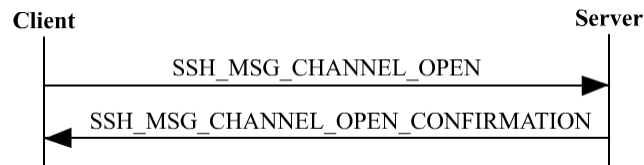
Figure 4.8: After the key exchange and user authentication phases, a channel can be opened, and data transfer can begin. Channels can be opened from either side.
