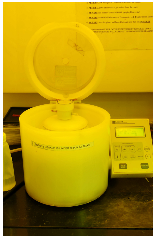
Figure 3.13 Laurel Technologies spinner in fume cupboard within yellow room.
