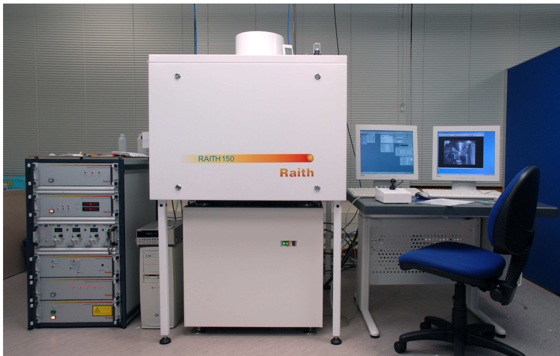
Figure 3.1 The ECE department's Raith 150 electron beam lithography system. From the left: a rack contains the control electronics and laser interferometer source; the Raith computer; the vacuum chamber of which the beam column can be seen extending through the top; the workstation of which the joystick stage control can be seen in front of two screens: one connected to the Raith computer and the other connected to the Leo computer controlling the Leo electron microscope.
