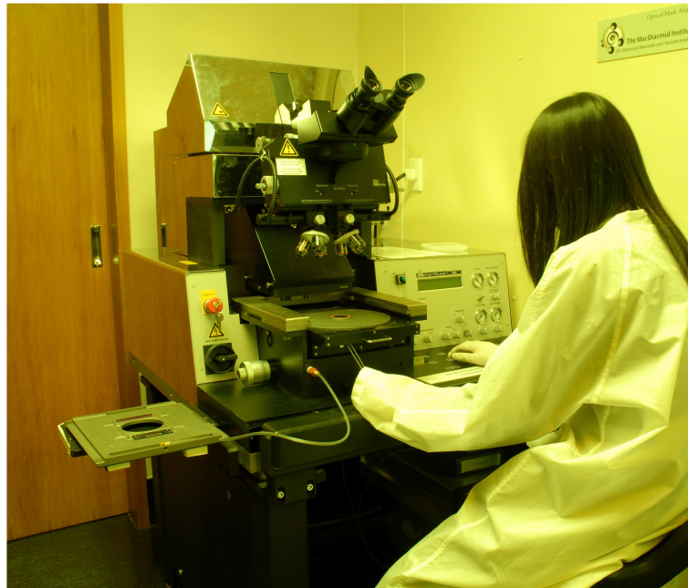
Figure 3.8 Karl Süss MA6 mask aligner with operator in the yellow room of the ECE micro-fabrication laboratory.
