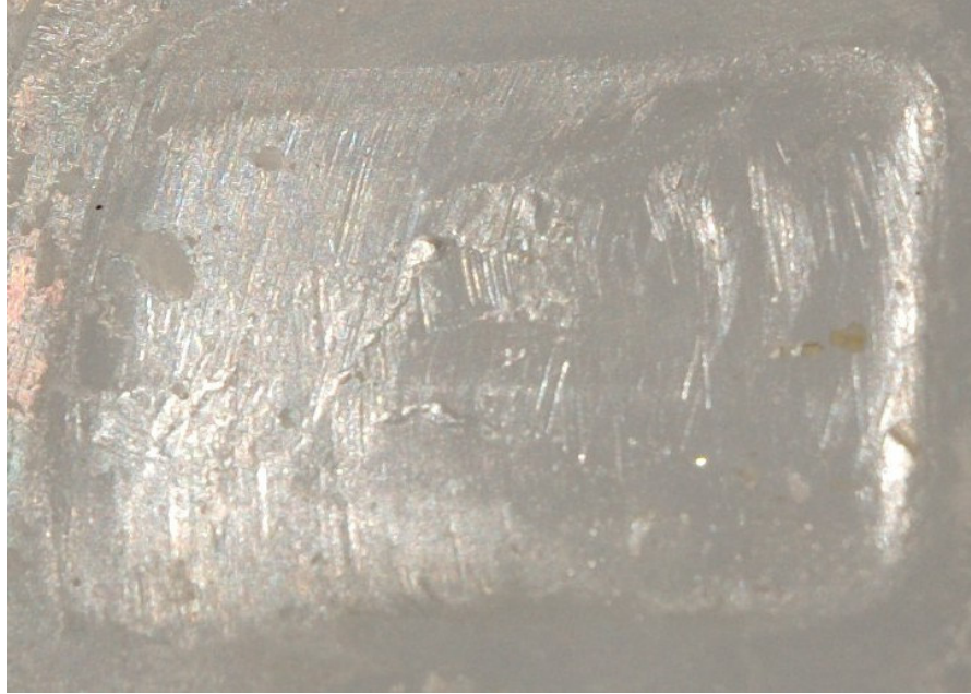
Figure 5-3 Close up of the wear track. Note the wear marks crossing each other
