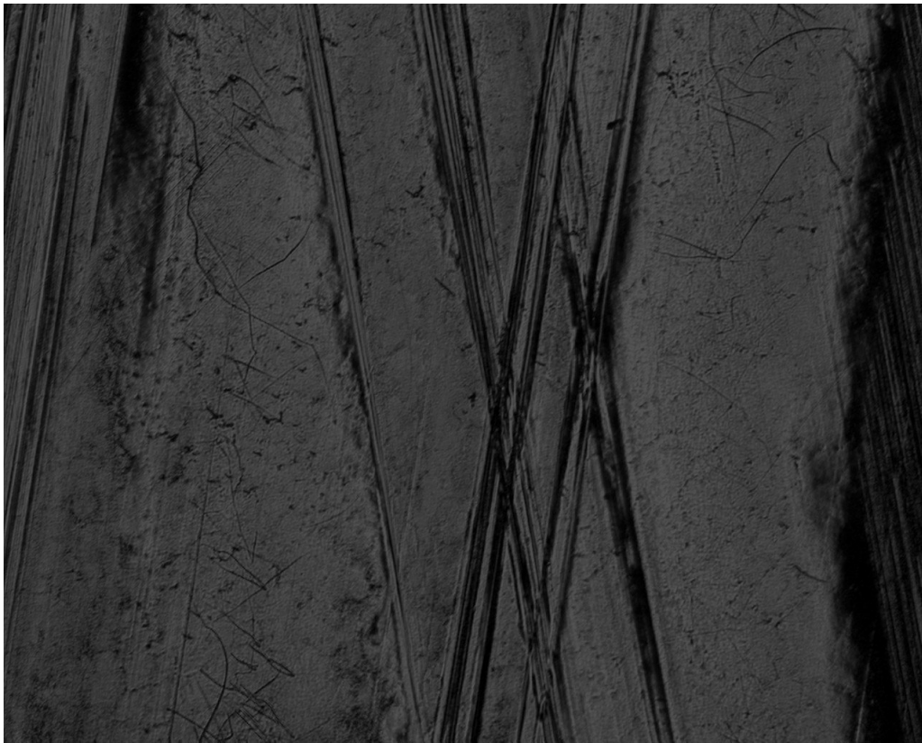
Figure 5-9 Gouge from sample 1. Original magnification 5x
