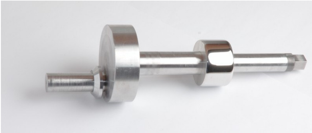
Figure 4-15 The completed FE shaft with femoral component
