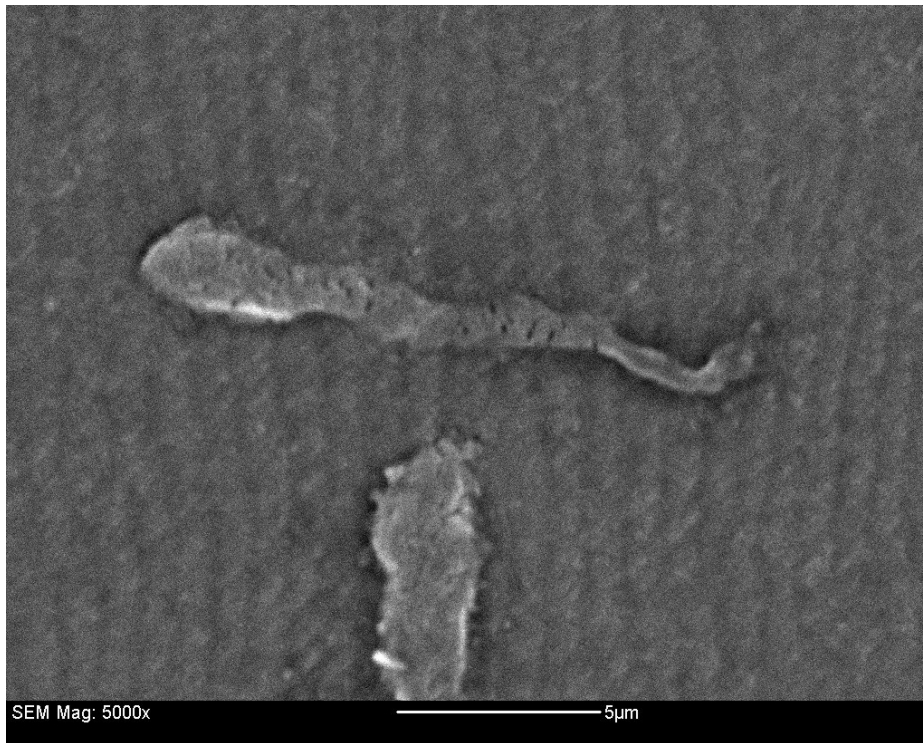
Figure 5-19 Embedded wear debris
