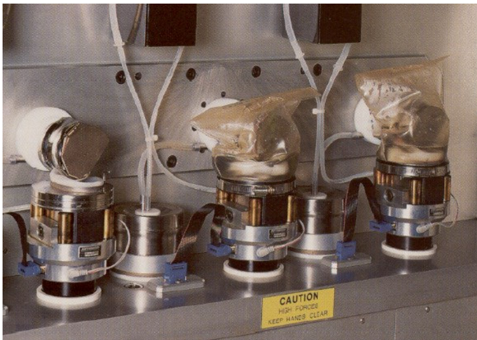
Figure 2-16 The AMTI KS2-6-1000 six station knee joint simulator
