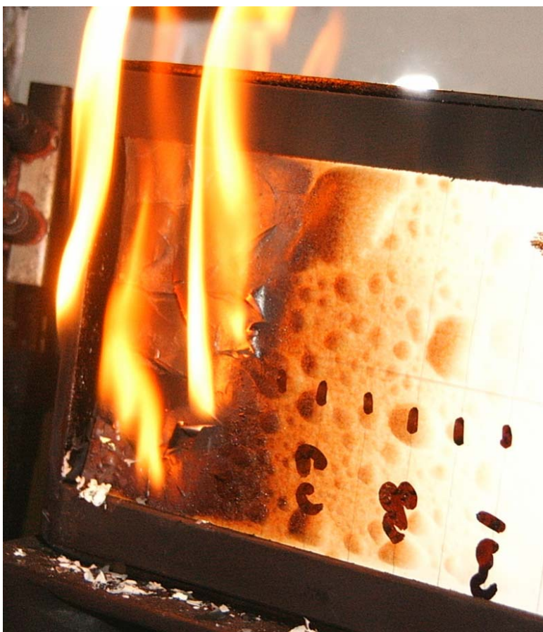
Figure 88: Flame spread behaviour of Melteca faced board
