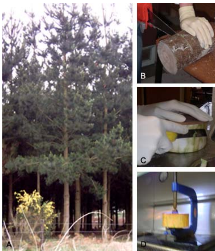
Figure 3.1 Sterilization technique. (A) Radiata pines planted in 1994 were felled, and stem segments were returned to the laboratory. (B) Discs approximately 10 cm in length were cut from the stem, following a series of washes (C) the outer rhytidome was removed, and the disc was (D) flame sterilized.
