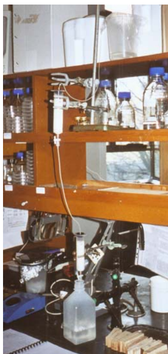
Figure 9.1 Ion-binding column set up. The concentrated culture media (top) was passed through two columns in tandem and collected in polypropylene containers (bottom).
