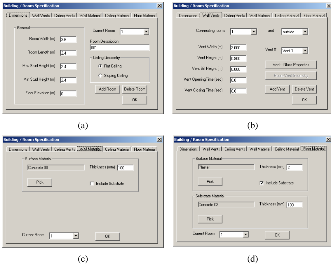
Figure 5. BRANZFIRE Room Design windows for the ISO 9705 test building (a) room dimensions; (b) wall vent; (c) wall material (d) floor material.
