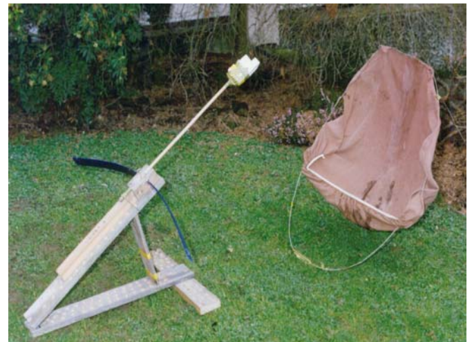
Figure 1: 1 st Example of Egg Launching/Catching System
