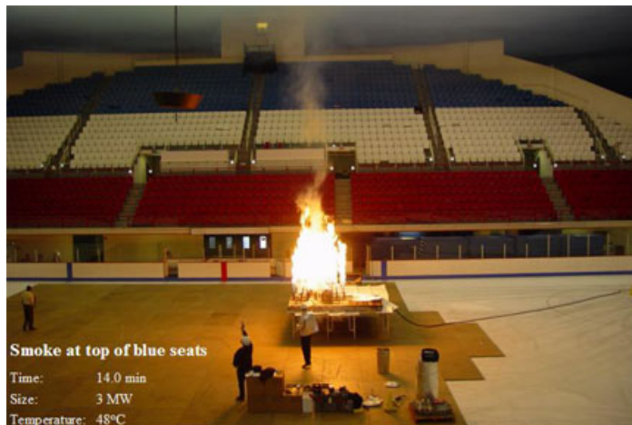
Figure 6 A hot smoke test in a sports arena [27]
