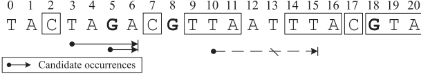
Fig. 7. Algorithm PMNS: checking candidate occurrences of the RE Q = (G|T)A^*GA^*T^* using PNS patterns and necessary factors, which are shown in bold font.
