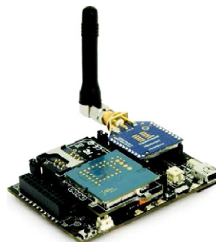
(b) Wasp mote sensor node with XBee-802.15.4
