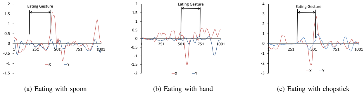
Fig. 4: Variation of the roll and pitch of gyroscope for various modalities of eating
