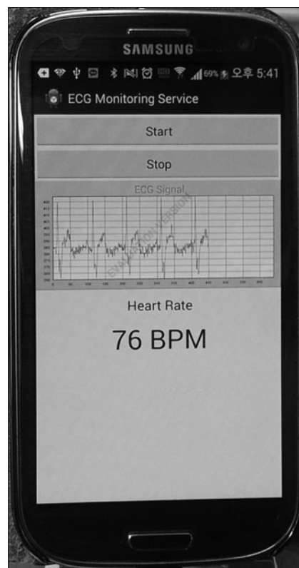
Fig. 4. A screenshot of the example healthcare application. The application shows the electrocardiogram (ECG) waveform and heart rate of the user in real time. BPM, beats/min.
