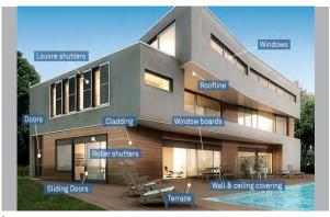
Fig. 2: Typical exterior applications of plastic based materials in contemporary buildings (Source: Inoutic, 2018)
