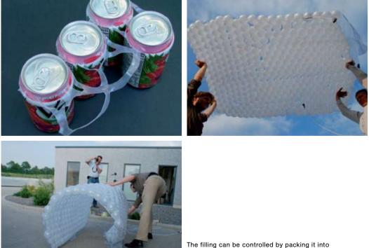
pre-manufactured units. Connecting elements made of punched plastic sheets, known from can pallets, could be used.
