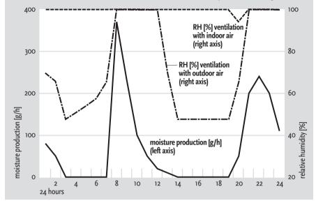
Figure 5.3 Moisture production PR and relative humidity in the bathroom, ventilation with outdoor and indoor air, calculated on the basis of the moisture production in Figure 5.2
