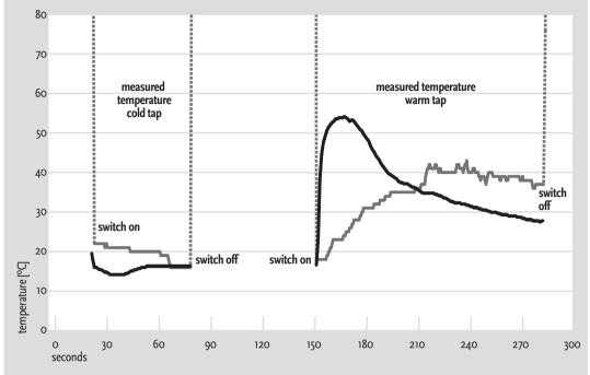
Figure A2.6 Typical representation of the measured water temperatures in the 364 sub-dataset on domestic cold and hot water
