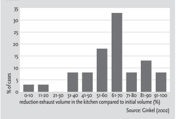
Figure 5.6 Total % of reduction in exhaust volume in the monitored cases
