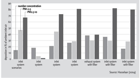
Figure 7.13 Deposition in the system, including HRU, based on experiments in the International Labatory of Indoor Air Quality and Health, Brisbane
