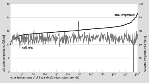
Figure 7.11 Cold (left axis) and hot (right axis) water temperatures of the subset on domestic water systems (n=364)
