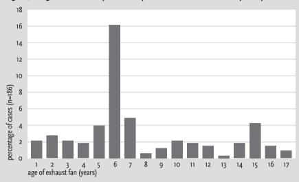
Figure 7.2 Age of the fan box (exhaust fan) in the sub-dataset on mould (n=186)
