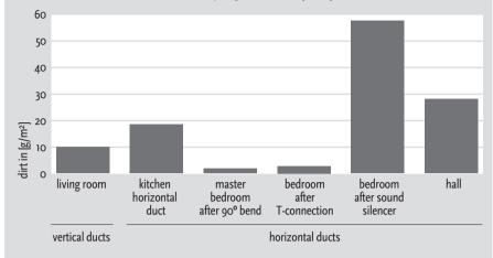
Figure 7.15 Deposition mass in ducts of balanced flow ventilation systems after 16 years, based on the sub-dataset on dust sampling in Arnhem (n=19)
