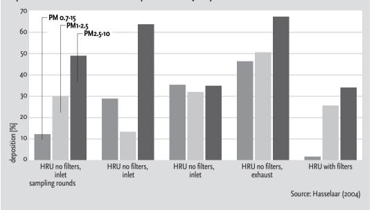
Figure 7.12 Deposition in heat recovery unit in scenarios that represent one period of sampling, based on experiments in the International Labatory of Indoor Air Quality and Health
