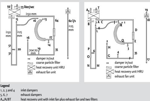
Figure A2.3 Layout and typical air velocities [l/s] in the figure on the left and sample points of the experimental design in the figure on the right
