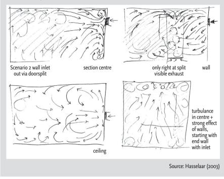
Figure 7.16 Air circulation patterns and particle movements in the test chamber at ILAQH, made visible by smoke: mechanical inlet from the wall and natural outlet via the door
