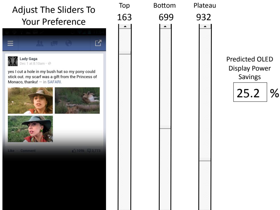
Figure 7.4: VBA Tool for user to control amount of dimming to be deployed
