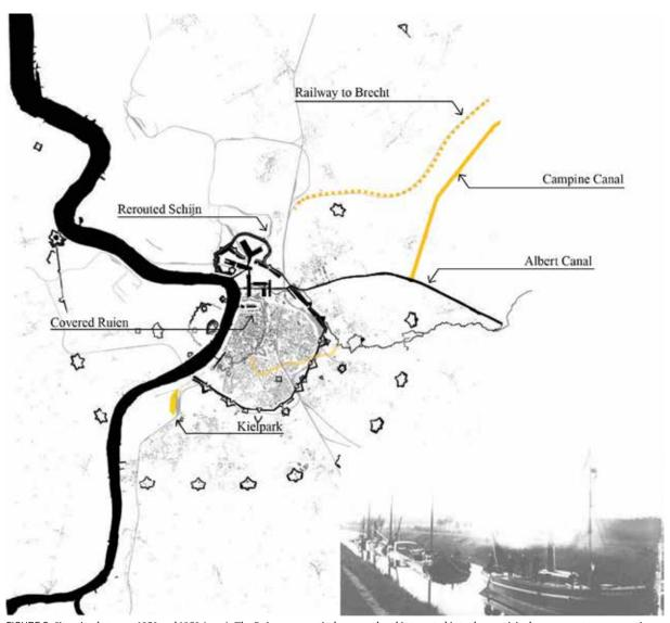
$FIGURE\ 3\ Situation\ between\ 1850\ and\ 1950\ (map).\ The\ Ruien\ were\ entirely\ covered\ and\ integrated\ into\ the\ municipal\ sewage\ system,\ evacuating\ waste\ water\ in\ the\ Scheldt\ River.\ Waste\ was\ transported\ to\ the\ countryside\ via\ the\ Campine\ Canal\ (1885-1916)\ (picture)\ and\ railway\ network.$
