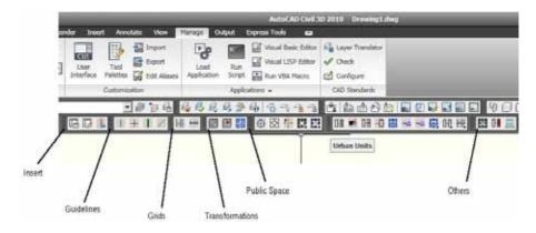
Figure 34 New toolbars with the CItyMaker tools.
