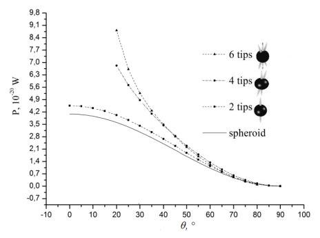
Figure 3. Dependence of the total absorption in the rotated AuNSt tip from its orientation with respect to the polarization vector of the light wave. Dashed lines show the results of Comsol calculations, solid - the dependence by the formula (1), where the volume of the spheroid multiplies U.
