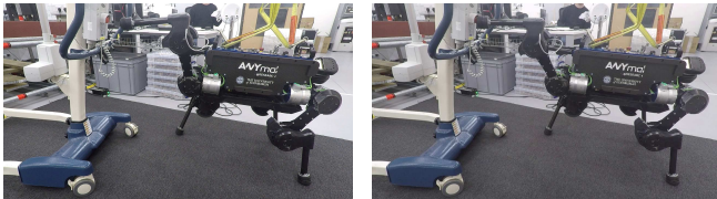
Fig. 3. Teleoperating ANYmal to press the e-stop button of a crane.
