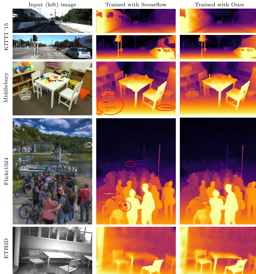
Fig. 6: Qualitative Results. Comparing our synthetic data generation approach with Sceneflow, using a PSMNet model trained on both. Our predictions benefit from semantically plausible depths at training time and have fewer artifacts.
