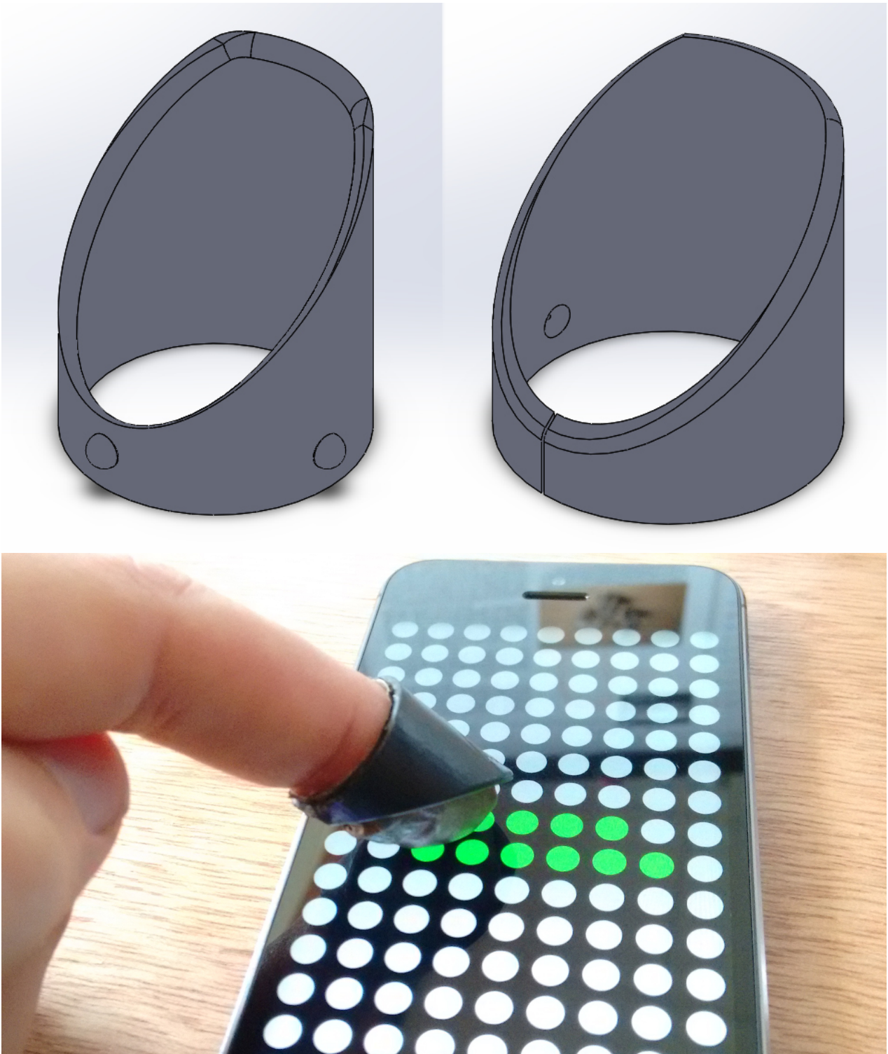
Figure 3. Second Iteration: Image (a) above showing the computer-aided design (CAD) of the second iteration of our touchscreen thimble , consisting of inner and outer cylinders that hold the conductive fabric in between. Photo (b) below showing the a Stereolithography (SLA) resin 3D-printed version of the CAD, in use on a capacitive touch smartphone.
