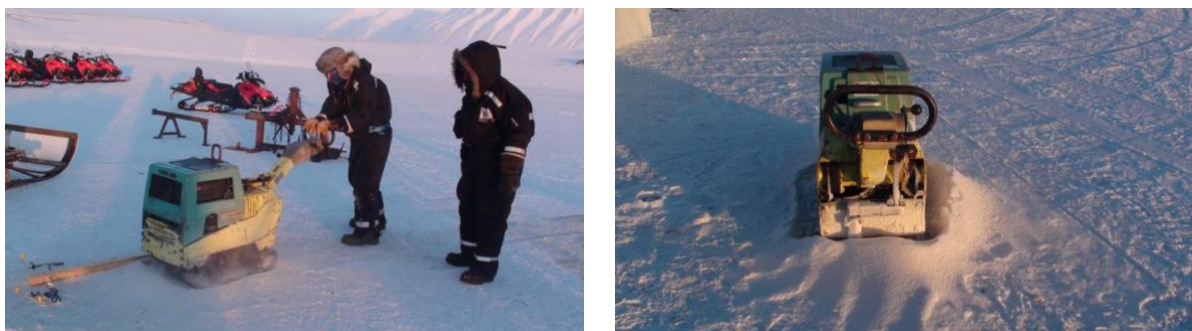
Figure 1. Vibrating plate on ice (left pane). Pulverization of ice surface by vibrating plate (right panel).
