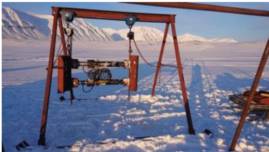
Figure 3. Hydraulic rig for indentation tests.
