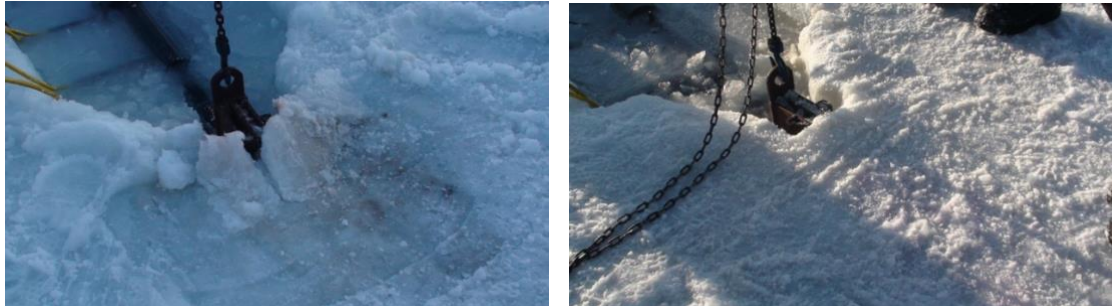
Figure 4. Indentation tests in the ice subjected to VP action (left panel) and in natural ice (right panel)
