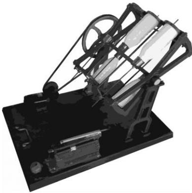
Fig. 2. Photo of custom-made equipment used for washing and soaking of horse rawhide.
