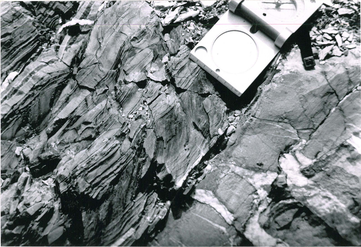
Figure 13: Intrabed cleavage formed easily in muddier laminations of finer dominant grain sizes.
