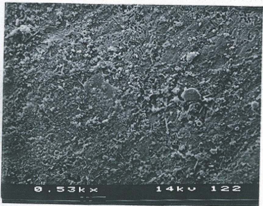
Figure 35: SEM image of claw dissolution at the 183 m site
