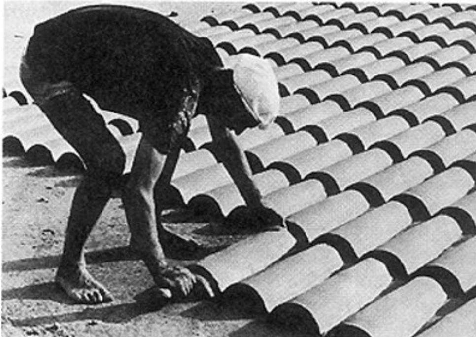
Figure 4: A modern tile-maker laying out imbrices to dry. (From Brodrigg, Roman Brick and Tile.)
