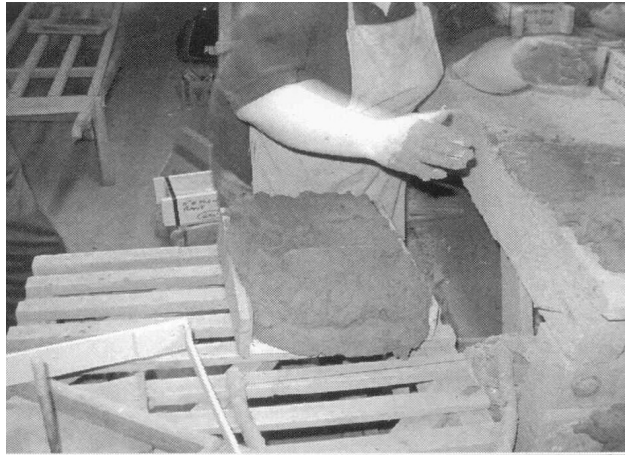
Plate 2.40: Loading clay into three-sided Mould C
