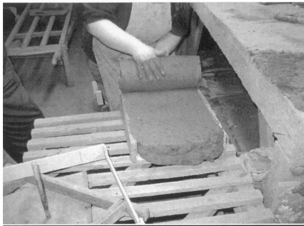
Plate 2.41: Peeling clay off mould after wiring
