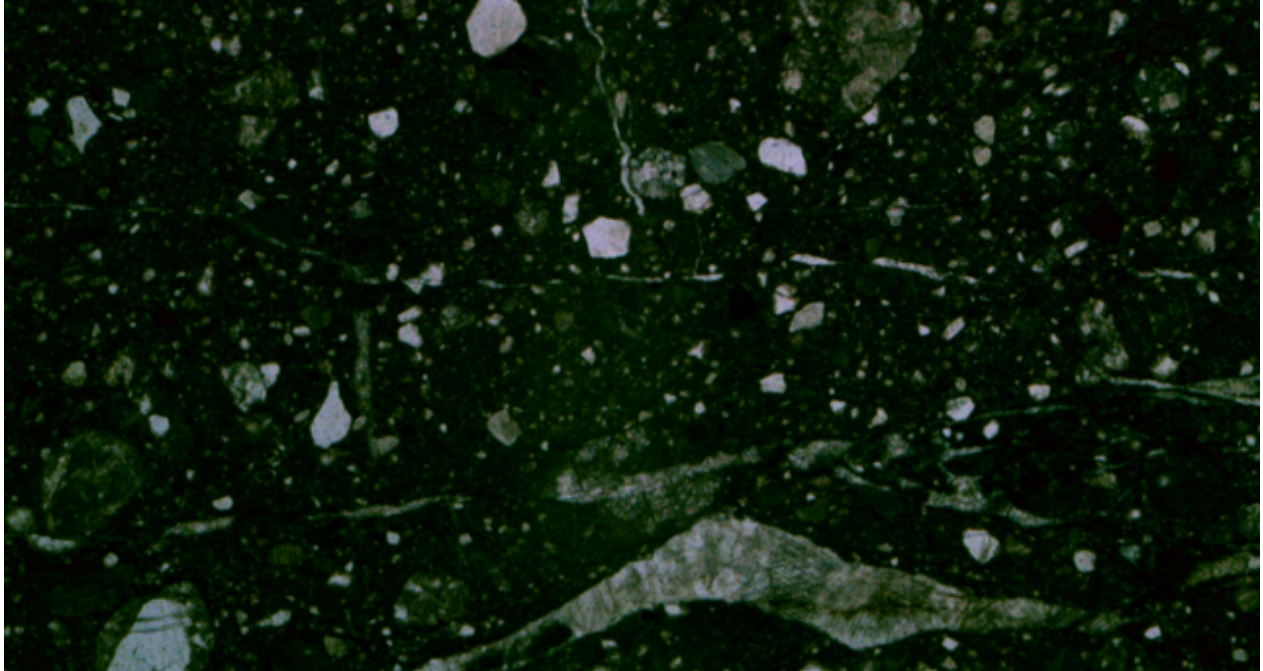
Figure 8: Thin section photomicrograph of Hunter Valley Fault rock; image width represents approximately 3 mm
