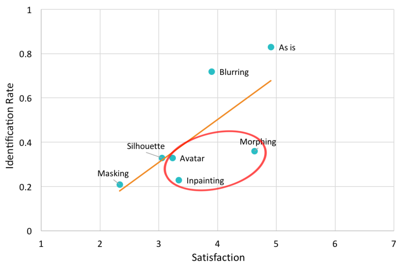
Figure 5.9: Scatterplot of Satisfaction (X axis) against Identification Rate (Y axis) which shows the general trade-off between effectiveness and satisfaction. Morphing , inpainting and avatar are below the regression line, which means they are relatively effective and satisfying.
