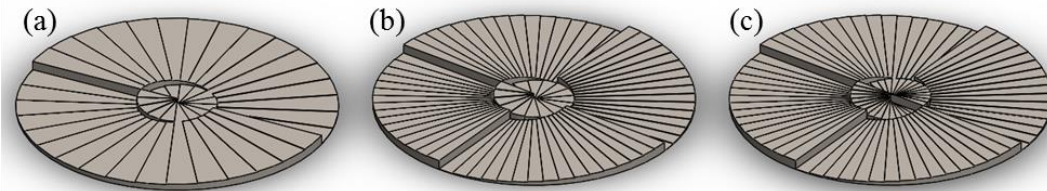
Figure 2.2.1 Schematic drawing of the concentric DPPs with (a) m_1 = 1 and m_2 = -2 (b) m_1 = 1 and m_2 = -4 and (c) m_1 = 2 and m_2 = -4 .
