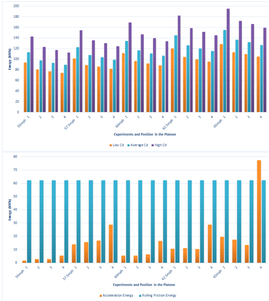
Figure 5.2: Energy consumption from aerodynamic drag (top) and acceleration and rolling friction (bottom) for different Speed
