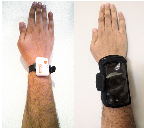
Figure 2.2: Photo comparing size of Shimmer3 with iPhone mounted on the wrist.
