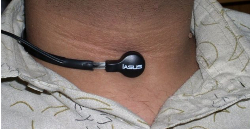
Figure 1.8: Throat microphone configuration used to detect swallowing in work by Sazonov et. al [38]
