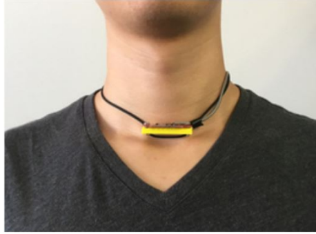
Figure 1.12: Proximity sensor employed by [57] to detect periods of eating from jawbone movement.
