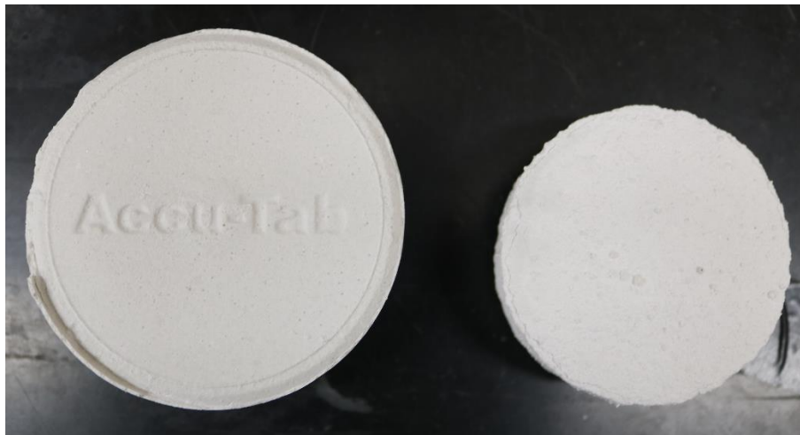
Figure 52. Chlorine tablet before and after one of the dissolution tests occurring over 7 hours.
