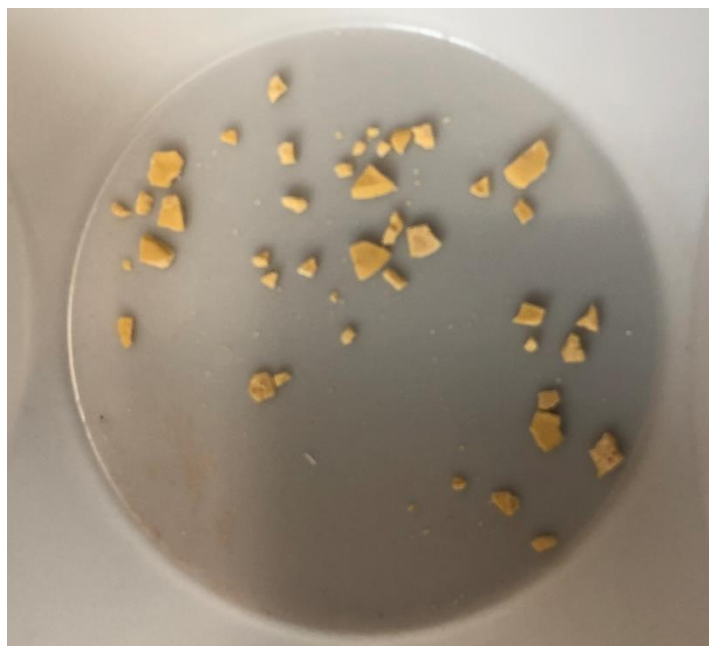
Figure 3-4 Photograph of melted aluminum doped LLZO pellets
